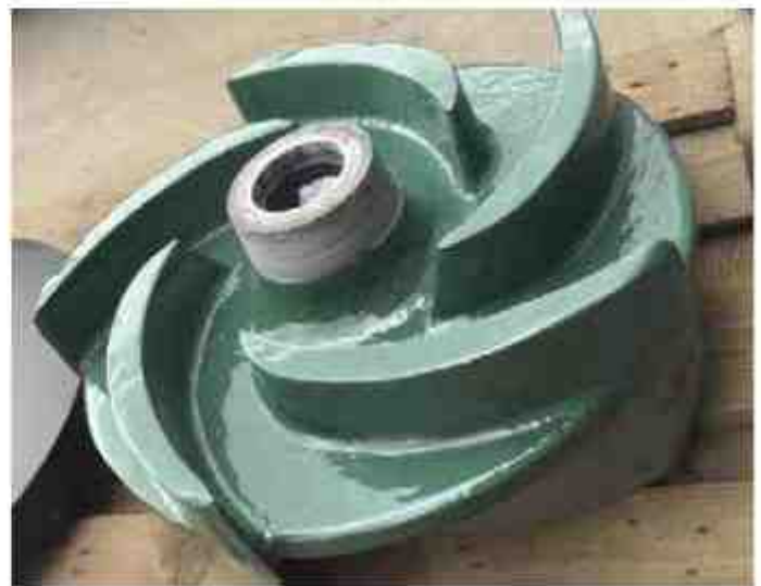
Pump impeller after repair with Loctite Wearing Compound, and PC 7255 Sprayable
