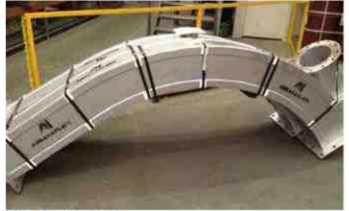
Chip Transfer Chute
